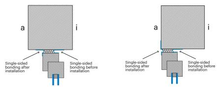
Examples: On the inside of the window (on the right in the picture), the tape was stuck to the window frame before the window was installed; on the outside (on the left in the picture), after the window was installed.
