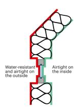
A building connection will retain its function in the long term if the layer on the inside and the windtight and driving rain impermeable layer on the outside are joined permanently and without gaps. This requires the creation of a sealing system with sufficient freedom of movement.
