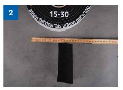
> Thickness of Ampacoll® Komprimax when not under tension.
