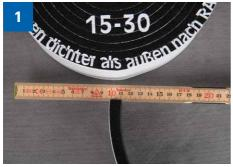
> Pre-compression: Ampacoll® Komprimax thickness immediately after opening of the roll.
