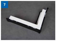
> Window frame prepared for installation. In the corner area, allow the strips to protrude. When attaching strips, also allow for extra length (create wave).
